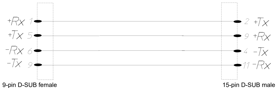
Fig. 10-1: Pin assignment for RS 485 interface cable for Anaprog controllers
