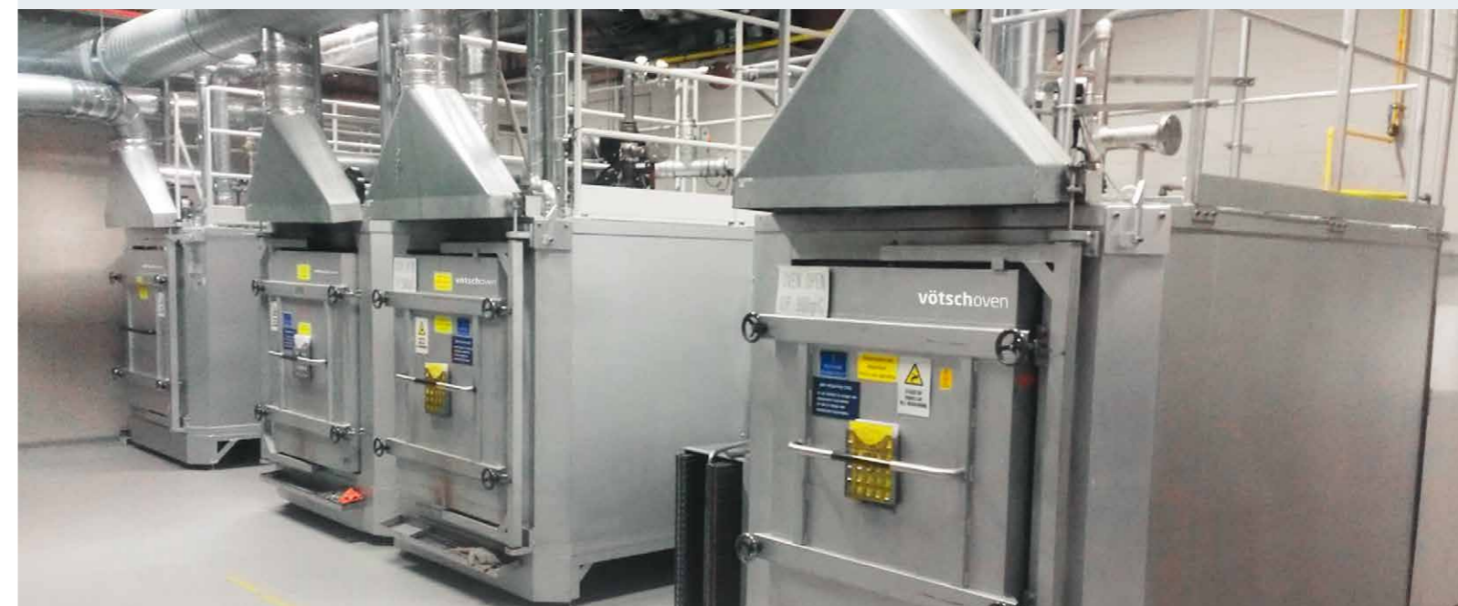
Annealing Furnace VAW 100/100/200-G-500 °C for the stress-relieving of welded constructions
