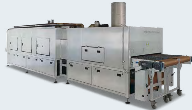
Curing Oven VDL 130/15/400-200 °C for medical products
