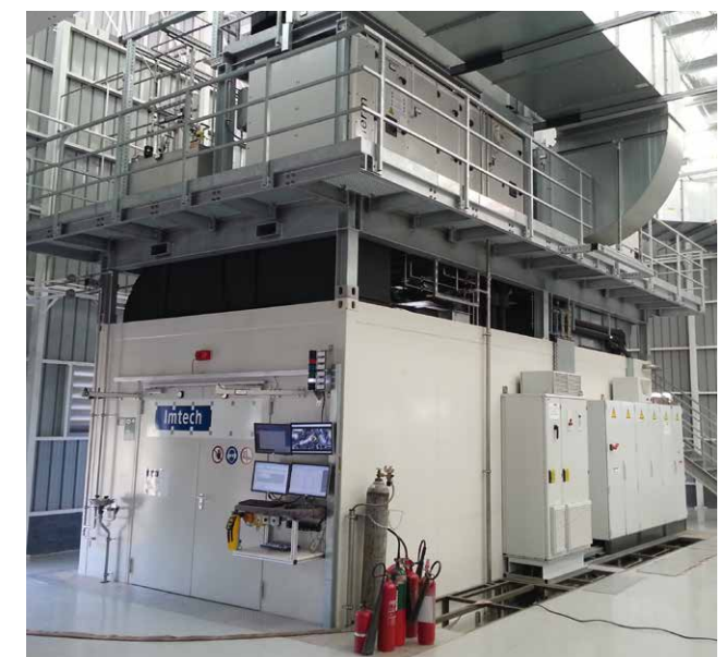
Test Bench Module with mounted supply frame
